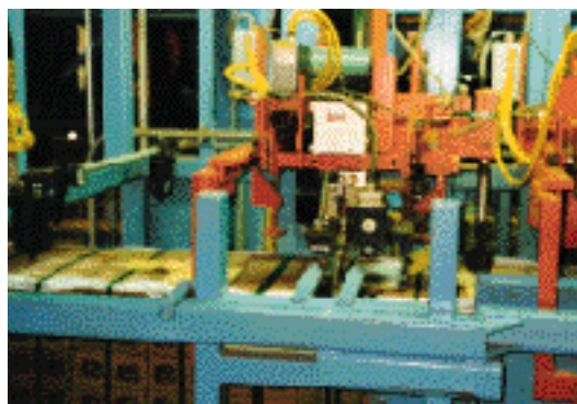
General Shale's automatic brick packing system.
