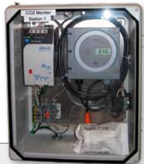
One of the Vaisala CARBOCAP® Carbon Dioxide Transmitters GMT222 used at the Chateau St. Jean winery.
